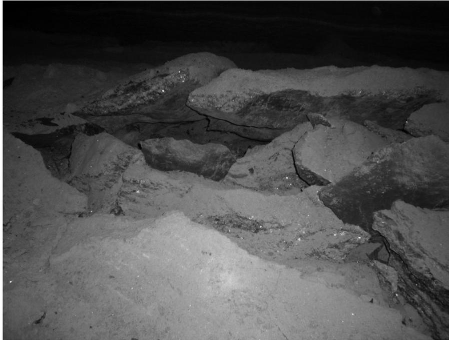
**Figure 1** - Rockburst in the sudden destruction of the rock floor, accompanied by gassing at Mine 4 AB bed.
