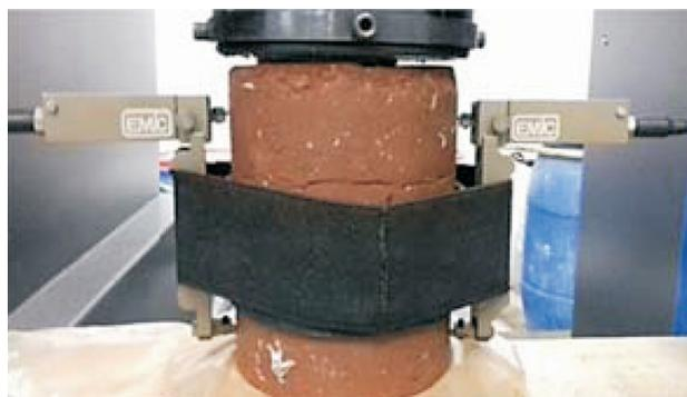
Figure 2 - Compressive strength with deflection control.
