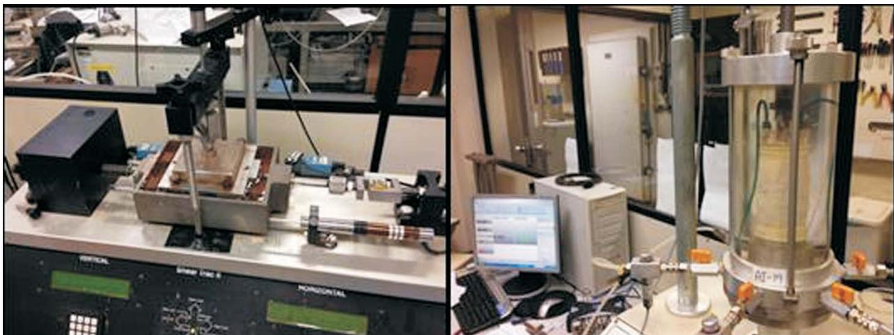
**Figure 8** - Conventional direct shear (left) and triaxial CIU (right).
