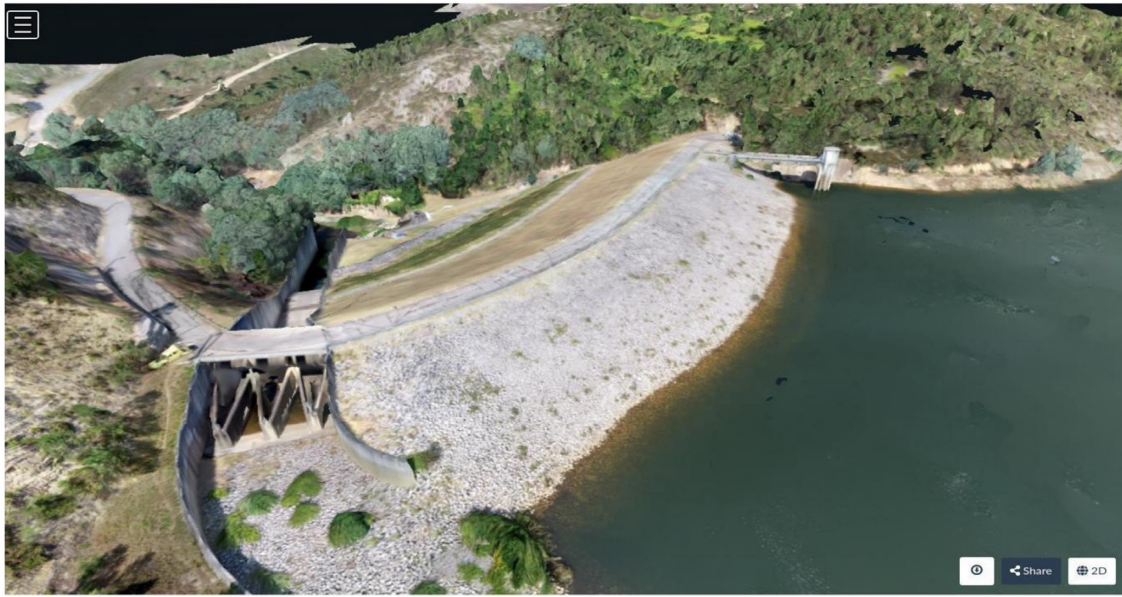
Figure 20. Textured model of the Lapa Dam (WebODM).
