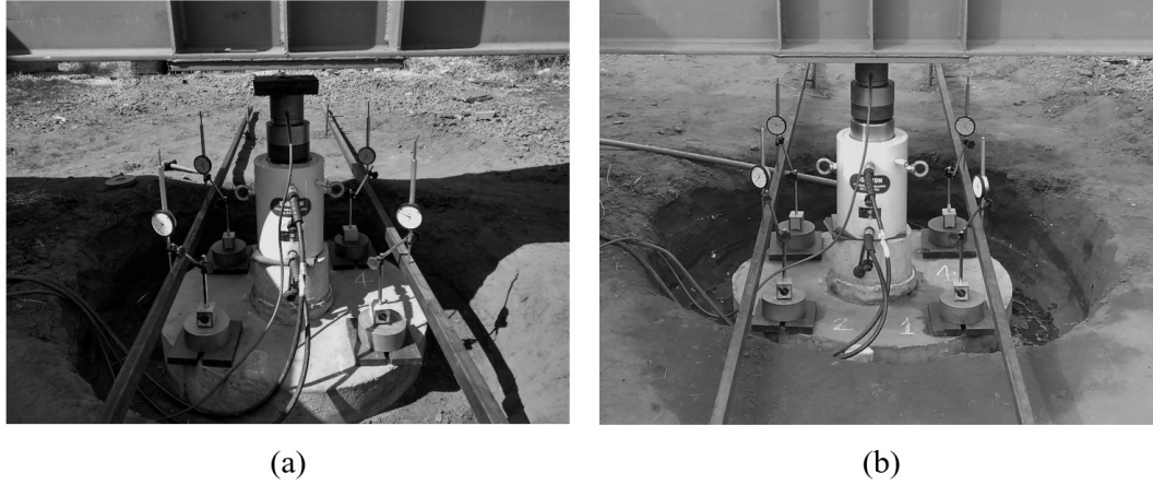
Figure 5. Loading test: (a) under natural conditions (LT-EXP-NAT); (b) under flooded conditions (LT-EXP-FLO).
