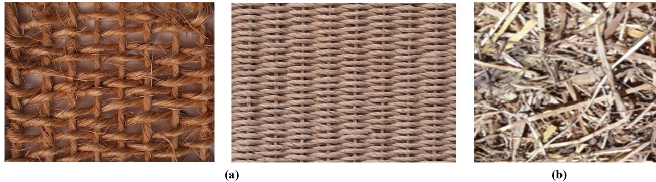
Figure 24. Examples of geosynthetics manufactured with natural fibres: (a) woven geotextiles from sisal fibres (courtesy J.R.M. Pimentel); (b) geomat for erosion control.
