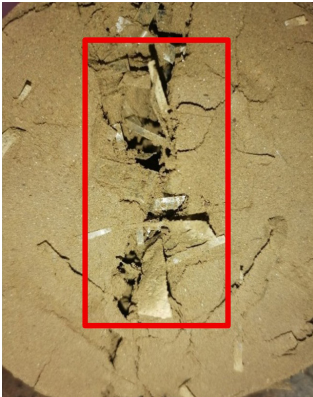
Figure 9. PWF along tension cracks (bridge action of PWF).
