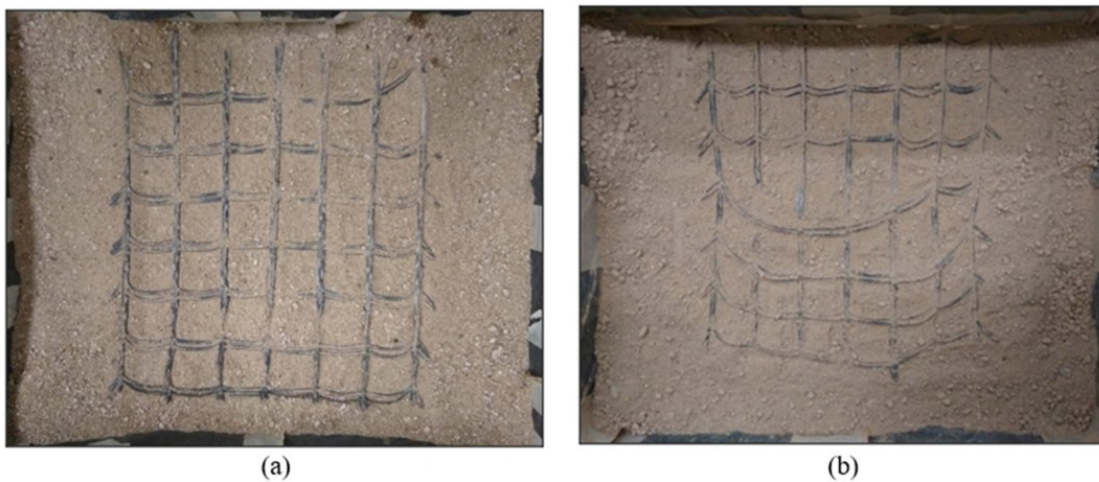
Figure 10. Exhumation of the geogrids used in the pull-out test ( \sigma = 50 kPa): (a) NS and (b) GRS-200-D.
