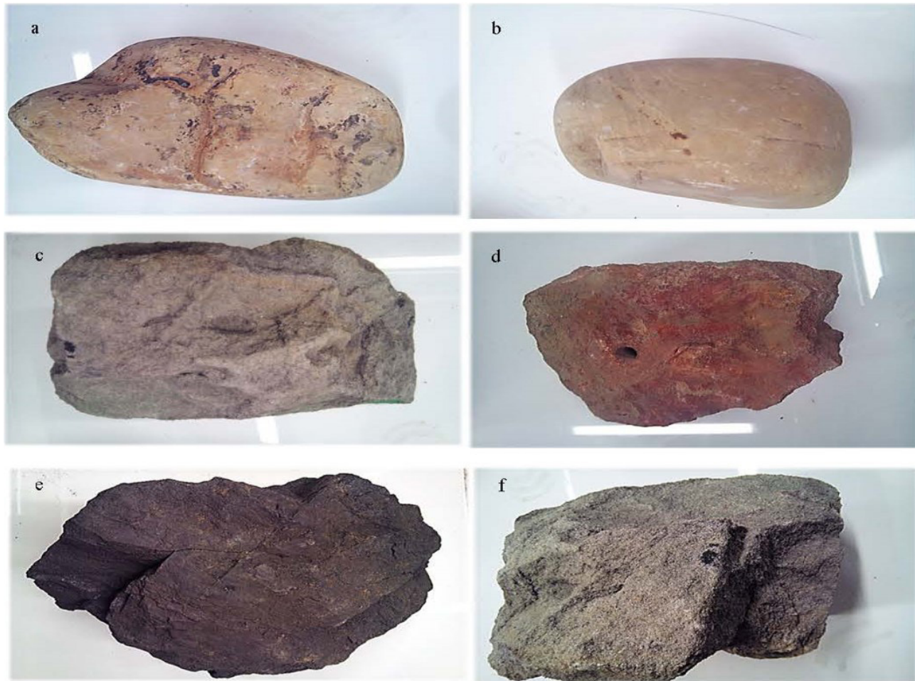
Figure 2. (a) Weak sandstone with faults from Table Mountain slopes, (b) Quartz from Table Mountain slopes, (c) Sandstone from Exarro, (d) Weak reddish weathered sandstone from Exarro, (e) Shale from Exarro, and (f) Sandstone from Exarro.
