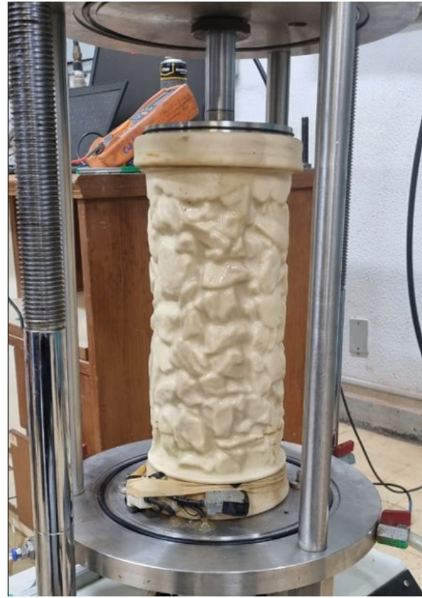
Figure 3. Specimen prepared for monotonic triaxial tests.
