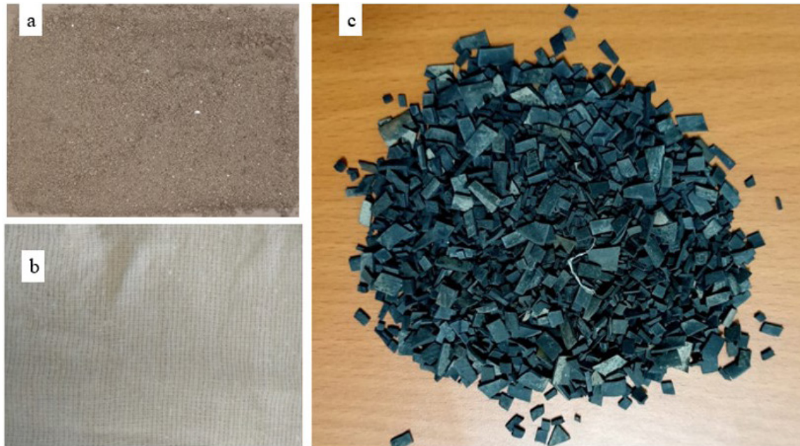
Figure 1. Photographs of material used: (a) sand; (b) geocell material; and (c) rubber.
