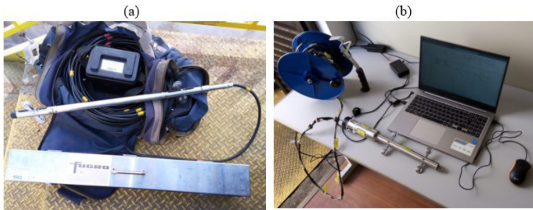
Figure 13. Inclinometer probes used: (a) Digitilt Datamate II; (b) experimental probe coupled to a notebook.
