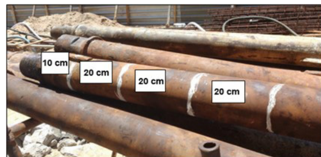
Figure 3. Marked sections on the last meter of the drilling rod.
