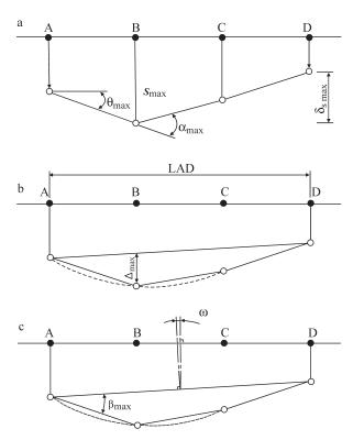
a) definitions of settlement *s*, differential settlement  $\delta s$ , rotation  $\theta$  and angular strain  $\alpha$ .
