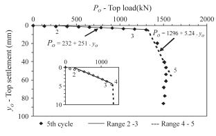
Figure 25 - Ranges 2-3 and 4-5 of the  $5^{th}$  cycle of loading - C1 Pile.
