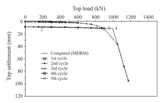
Figure 23 - Load-settlements curves from the static loading test on Pile T1, with modelled (by MDRM) curves for the  $5^{th}$  cycle of loading.
