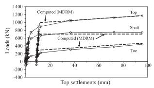
Figure 24 - Measured and computed (by MDRM) loads - T1 Pile ( $5^{\text{th}}$  cycle).
