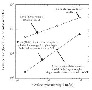
**Figure 13** - Comparison of leakage rates for GM/CCL composite liner and a range of interface transmissivities as calculated from analytical solutions and FEM analysis for (a) a single hole in direct contact with the GCL and (b) a single 15 m long wrinkle with a hole.  $k_L = 5 \times 10^9$  m/s,  $H_L = 0.51$  m, L = 15 m, B = 30 m and 2b = 0.3 m.
