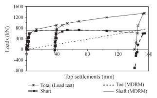
Figure 21 - Computed shaft and toe loads - E9 pile.
