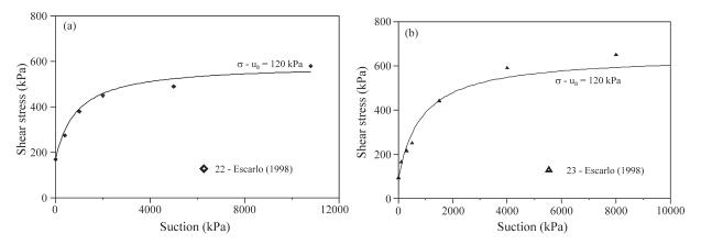
Figure 5 - Experimental and predicted shear strength envelopes considering one set of tests with dry samples. (a) Madrid gray clay. (b) Guadalix red clay (data from Escario, 1988).
