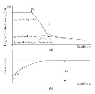
**Figure 2** - (a) Soil water retention curve and typical elements; (b) Hyperbolic function and assumed conditions to derive a and b parameters.
