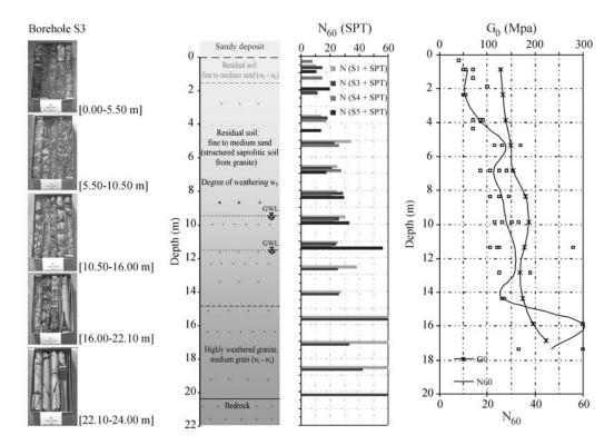
Figure 2 - Geotechnical profile with photos taken from samples obtained in borehole S3;  $N_{60}$  results in depth with average shear modulus  $G_a$  from CH shear waves, across two different sections: S2-S1 & S3-S2.
