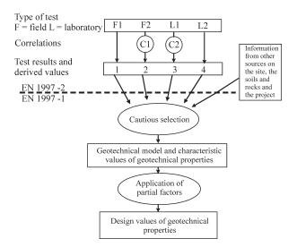
**Figure 1** - General framework for the selection of derived values, characteristic values and design values of geotechnical properties (CEN, 2006).
