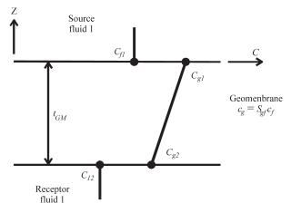
**Figure 14** - Concentration profile for diffusion across a geomembrane showing (a) partitioning between the concentration in the source solution,  $c_{jl}$ , and the concentration in the adjacent geomembrane,  $c_{gl}$ ; (b) diffusion profile from the top to bottom of the geomembrane; (c) partitioning between the concentration at the bottom of the geomembrane,  $c_{g2}$  and the concentration in the receptor solution,  $c_{g}$ . Note that  $c_{gl}/c_{gl} = c_{gl}/c_{gl} = S_{gr}$ .
