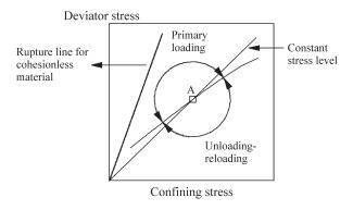
Figura 2 - Stress level and stress state criterion (after Duncan *et al.*, 1984).
