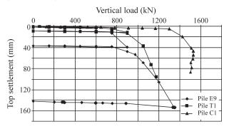
Figure 10 - Load-settlement curves from static load test.
