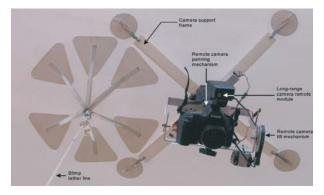
Figure 6 - Photograph showing digital camera mounted to the underside of the blimp (after Chappel *et al.* 2007).
