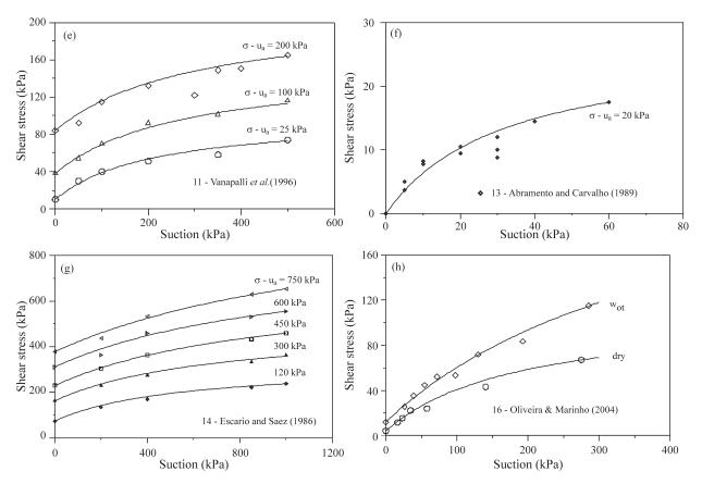
Figure 6e-h - Experimental and predicted shear strength of soils from Table 1, considering the effective shear strength parameters of saturated soil and the shear strength at the largest suction used in the tests.
