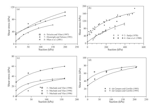
Figure 6a-d - Experimental and predicted shear strength of soils from Table 1, considering the effective shear strength parameters of saturated soil and the shear strength at the largest suction used in the tests.
