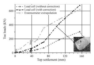
**Figure 13** - Comparison of the values of the load transmitted to toe in pile E9, deduced form the load cell without and with area correction and measures from the extensioneters.
