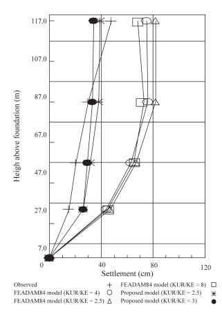
Figura 4 - Predicted and observed vertical displacement under Foz do Areia dam axis (Saboya Jr. & Byrne, 1993).
