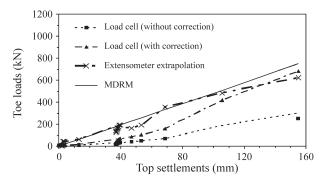
Figure 20 - Measured and computed toe loads.
