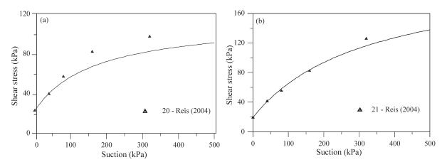
**Figure 4** - Shear strength envelopes of residual soil from gneiss and experimental and predicted variation of shear strength considering results of tests with air dried samples: (a) young soil; (b) mature soil (data from Reis, 2004).
