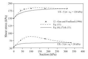
**Figure 7** - Ash tuff tested by Gan & Fredlund (1996) fitted with Eq. (12) and values predicted by Eqs. (6), (7) and (11).
