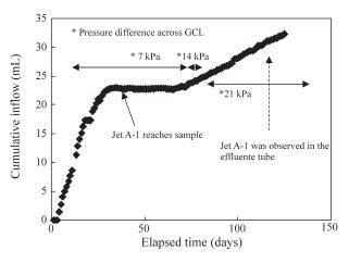
**Figure 1** - Variation in cumulative inflow volume through the GCL with time for a GCL subjected to 12 freeze and thaw cycles and permeated with water and Jet A-1 in flexible wall permeameter test (modified from Rowe *et al.*, 2005c).
