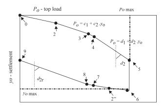
**Figure 17** - Theoretical load-settlement curve of pile head for  $A \neq 0$  - short piles.
