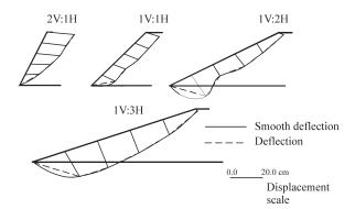
**Figura 9** - Deformed shape of the upstream face after the reservoir filling.
