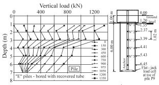
Figure 11 - Load distribution - measured in the  $5^{th}$  cycle of loading.
