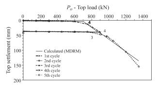
**Figure 19** - Load-settlements curves from the static load test on Pile E9, with theoretical curves for the 4<sup>th</sup> and 5<sup>th</sup> cycles of loading.
