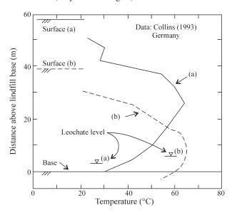
**Figure 2** - Temperature variation with depth at two locations, (a) and (b), in an old landfill (1936-1980) in Hannover Germany; waste circa 1938 at bottom (after Rowe, 1998).
