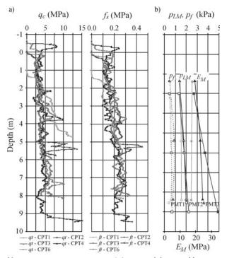
Note: pore pressures measurements  $(u_i)$  are zero: it is reasonable to consider  $q_c \equiv q_i$  and  $f_i \equiv f_i$ .
