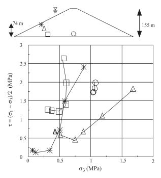
Figura 1 - Stress path during reservoir filling of Foz do Areia Dam (Saboya Jr., 1993).
