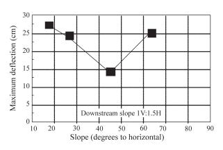
Figura 5 - Maximum deflection vs. upstream slope.
