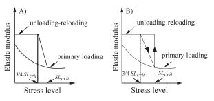
Figura 3 - Loading and unloading criteria: a) Proposed by Duncan *et al.* (1984); b) Proposed by Saboya Jr. & Byrne (1993).
