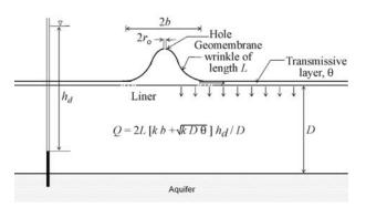
Figure 11 - Schematic defining leakage through a composite liner with a wrinkle. Assumes lateral migration at interface and vertical flow in clay liner.
