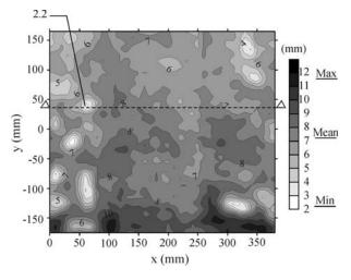
**Figure 9** - Contours of the final thickness of a GCL after application of 250 kPa vertical pressure. Configuration comprised (from top down) nominal 50 mm gravel, for a 2000 g/m<sup>2</sup> needlepunched nonwoven protection layer, geomembrane and GCL (w = 115%), sand layer (adapted from Dickinson & Brachman, 2006). Marked cross-section shown in Fig. 10.
