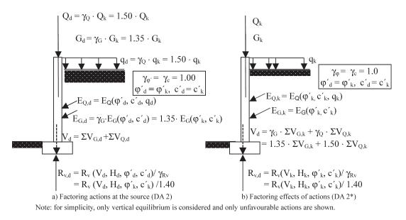
Figure 3 - ULS in p&tds. Design Approach 2 - introduction of partial factors (recommended values) in the verification of ground bearing capacity (Frank *et al.*, 2004).
