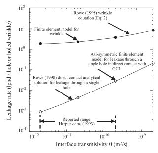
**Figure 12** - Comparison of leakage rates for GM/GCL/attenuation layer composite liner and a range of interface transmissivities as calculated from analytical solutions and FEM analysis for (a) a single hole in direct contact with the GCL and (b) a single 15 m long wrinkle with a hole.  $k_L = 5 \times 10^{-11}$  m/s,  $H_L = 0.01$  m,  $k_j = 1 \times 10^{-6}$  m/s,  $H_i = 0.5$  m, L = 15 m, B = 30 m and 2b = 0.3 m.
