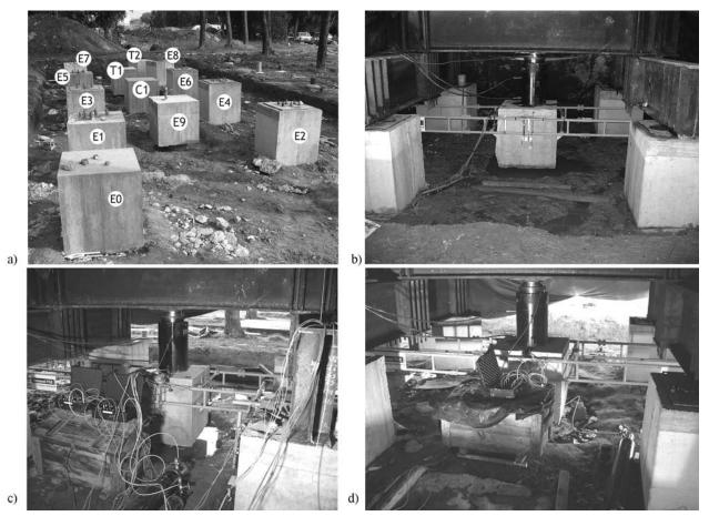
Figure 7 - a) Layout of the experimental site; pile tests: b) driven pile (C1); c) bored pile (E9); d) CFA pile (T1).
