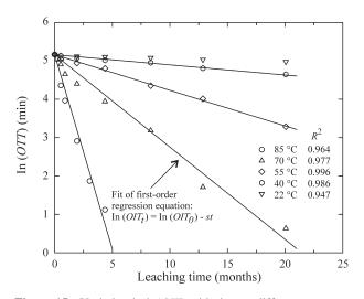
**Figure 15** - Variation in ln(OIT) with time at different temperatures in leachate.  $OIT_o$  is the initial OIT and  $OIT_i$  is the OIT at time *t* (month), s is the antioxidant depletion rate (month<sup>-1</sup>) (after Islam & Rowe, 2007).
