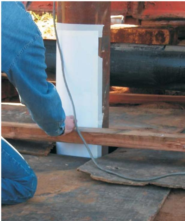
**Figure 7** - Settlement measurements using paper sheet and pencil.
