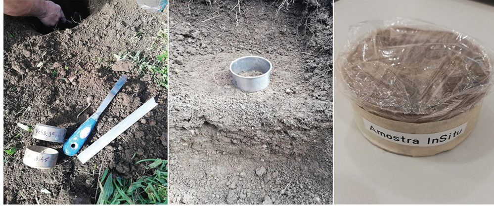
Figure 3. Extraction of undisturbed in-situ specimens.
