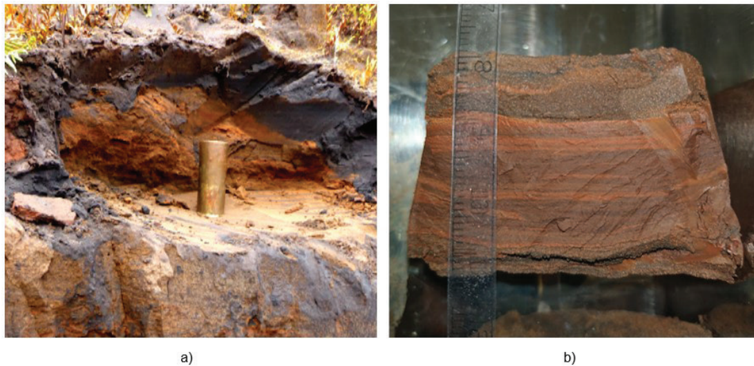
Figure 2. Examples of localised layer variability: (a) layering visible in the field; (b) micro layering, visible on an undisturbed sample from Site 1 (12/19/2019) at LabGEO.
