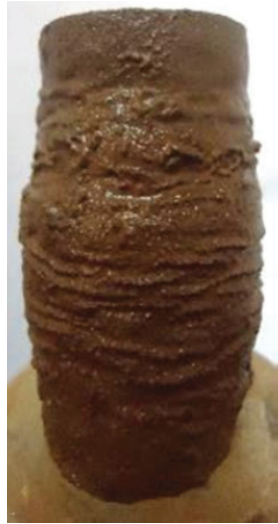
Figure 16. Photograph of the undrained triaxial test result of a loose specimen (~78%) of flotation tailings (BL-2&1).
