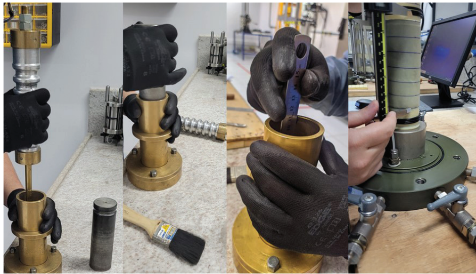
Figure 4. Dense specimen preparation method.
