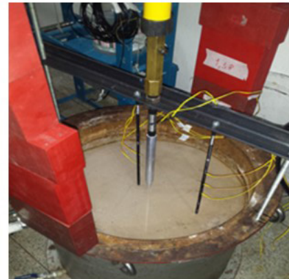
Figure 1. (a) lay-out of the container and instrumentation (b) torpedo and instrumentation installation.
