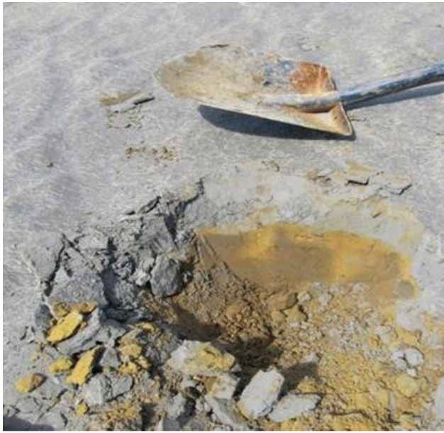
Figure 3. Thickened tailings with unoxidized layer overlying oxidized tailings.
