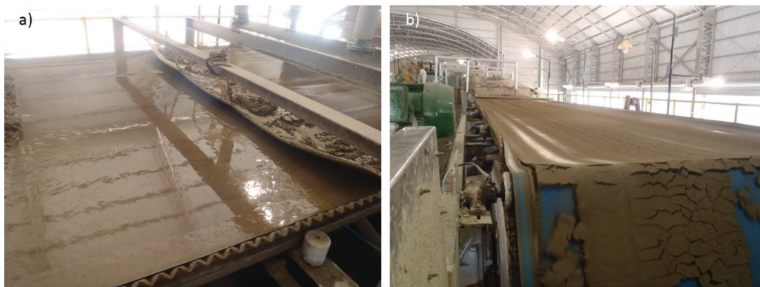
Figure 2. Vacuum belt filter at Casposo Mine. (a) Tailings being fed to the filter band; (b) Tailings at filter output.
