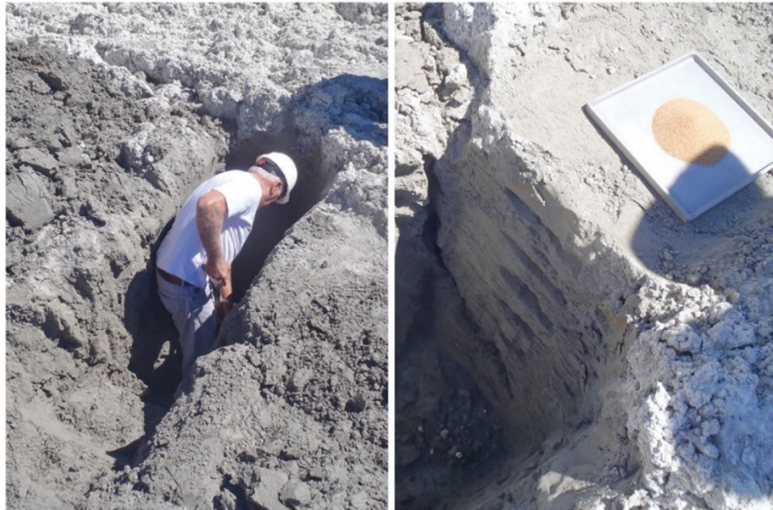
Figure 8. Exploration trenches dug in the upper tailings layer while exposed to the atmosphere.
