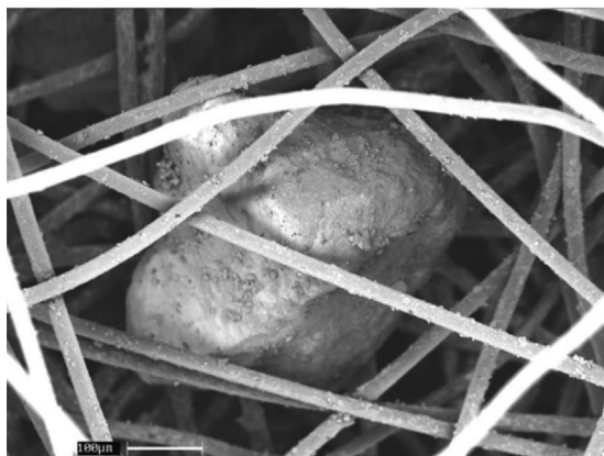
Figure 15. Entrapped soil particles in a geotextile filter exhumed from a drain in BR-020 highway (Gardoni, 2000).
