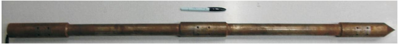
**Figure 2** - Photo of the seismic probe.
