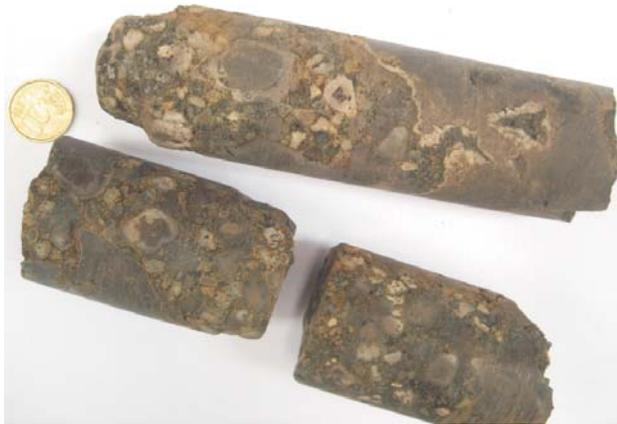
**Figure 22** - Hyaloclastite rock cores.
