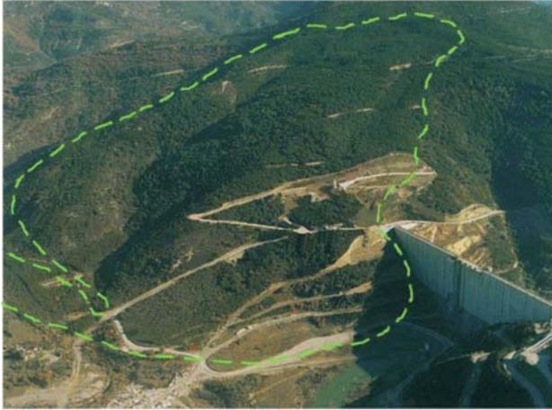
**Figure 7** - Paleo-landslides area near the Itoiz dam.
