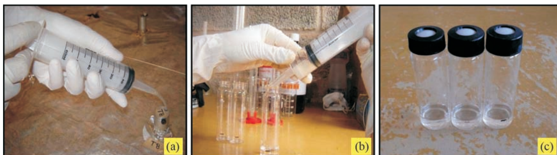
Figure 13 - (a) Introduction of the hose in the monitoring tube; (b) Injection of the contaminated solution in the vial; (c) Sealed vials.
