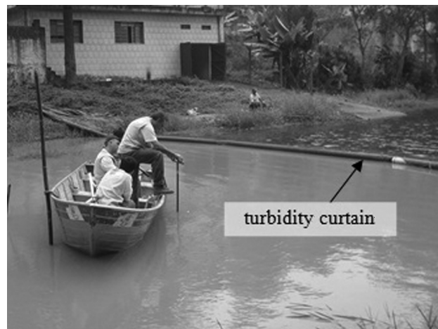
Figure 3 - Sediment sample being collected upstream of a turbidity curtain (3 rd BMP at drainage exit # 6) during the monitoring activities.
