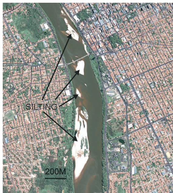
Figure 11 - Areas strongly affected by erosional processes and silting: a) sediment deposits (Site 32 - Fig. 5) in the Parnaíba River (city of Teresina - Piauí State) and b) gullies in the Camapuã region (northeast portion of Mato Grosso do Sul State, Site 38 - Fig. 5).
