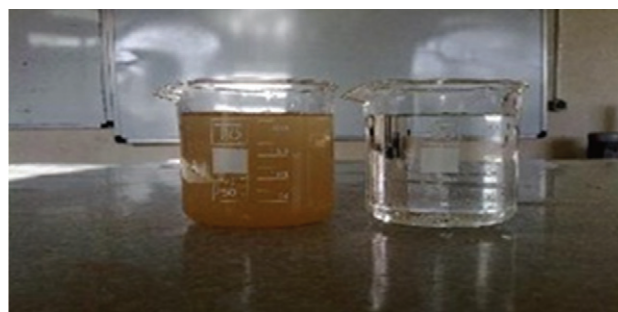
Figure 5 - Changes in the dispersive and non-dispersive soils discharged water.
