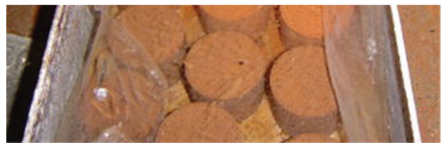
Figure 5 - Test specimens immersed cured.
