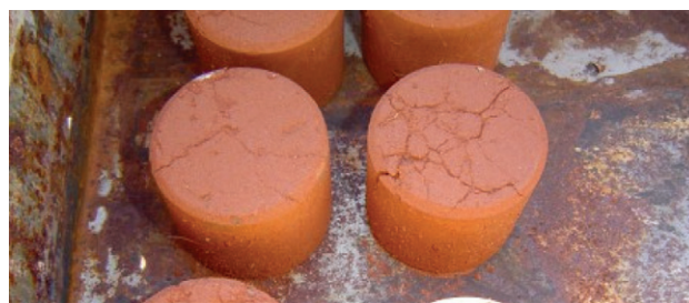
Figure 9 - Soil test specimens cured under full exposure.
