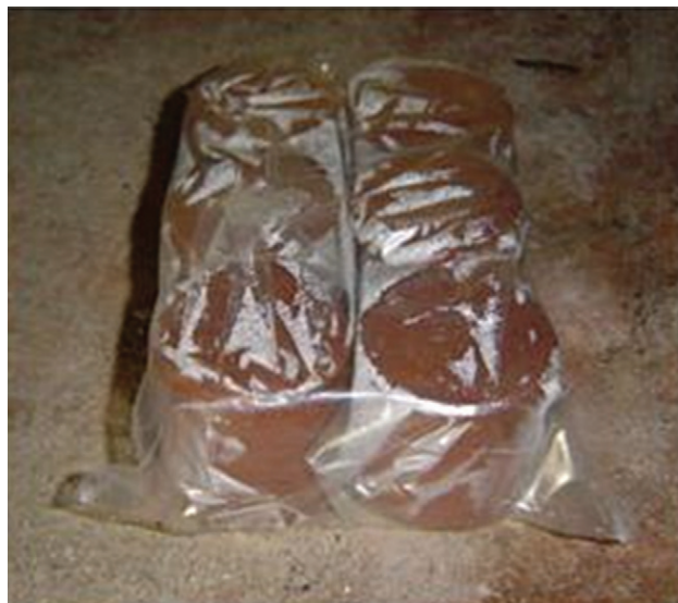
Figure 4 - Test specimens stored in a moist chamber.
