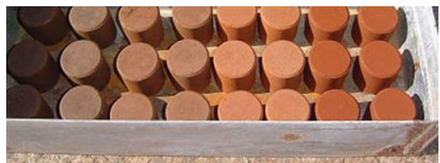
Figure 7 - Fully exposed cured test specimens.
