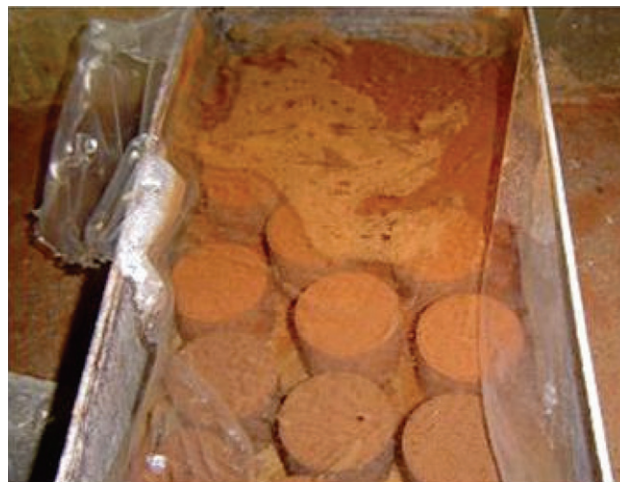
Figure 8 - Soil test specimens after immersion.
