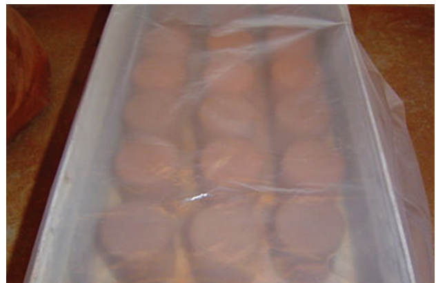
Figure 6 - Test specimens cured in a kiln oven.
