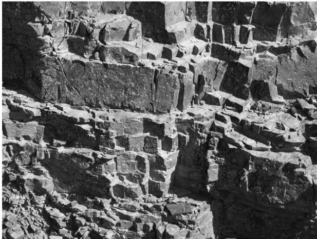
**Figure 8** - Lechago dam. Outcrop of Cambrian quartzitic shales quarried for rockfill material.
