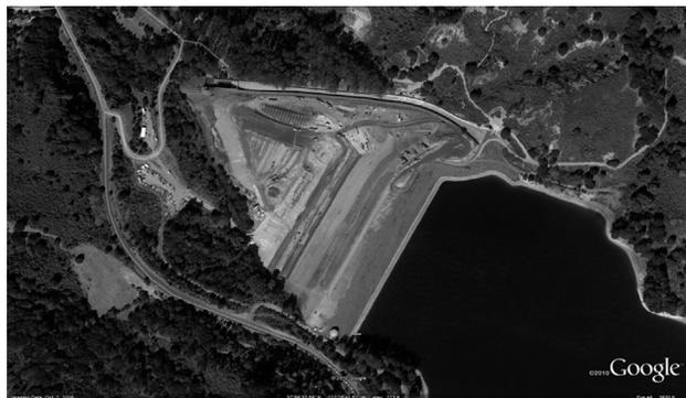
**Figure 5** - San Pablo Dam in 2010 after seismic remediation using cement deep soil mix in the downstream foundation and a downstream stability berm (Google Earth, Imagery Date 10/2/2009).
