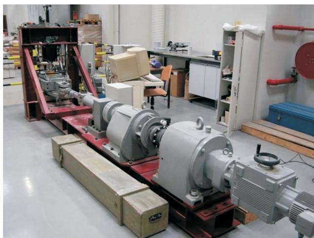
Figure 7 - Discontinuity shear tests.
