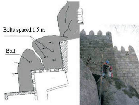
**Figure 22** - Plan of nailing positioning and drilling.
