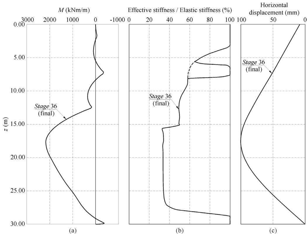
**Figure 36** - Results of the analysis considering the nonlinearity of the concrete wall at the completion of the excavation: a) wall bending moments; b) ratio between the effective and the elastic bending stiffness; c) lateral wall displacements.
