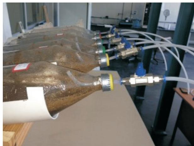
**Figure 3** - Batch reactors mounted on a shaking wood support, also showing valves used for periodic gas venting.
