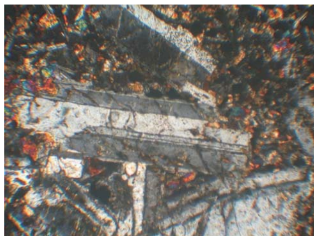
Figure 2 - Photomicrograph showing subophitic texture of basalt sample. Pyroxene crystals occur in an array with labradorite plagioclase in form of parallel laths. The polarized light (PL) field width is 1.5 mm.
