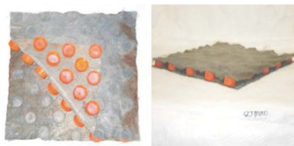
a) Drainage core consisting of PET bottle caps.
