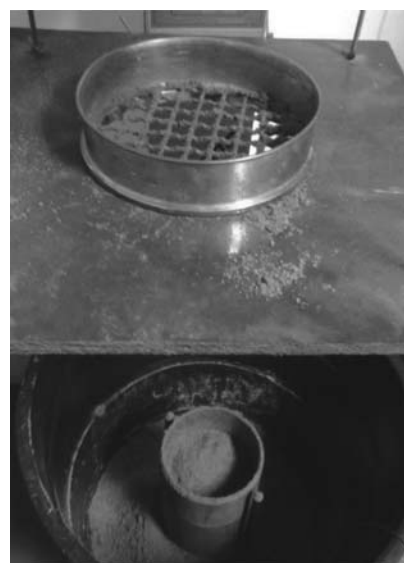
Figure 6 - Pluviation device used for molding the test specimens.
