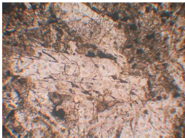
Figure 3 - Same rock section under nonpolarized light (NL) with a field width of 1.5 mm.
