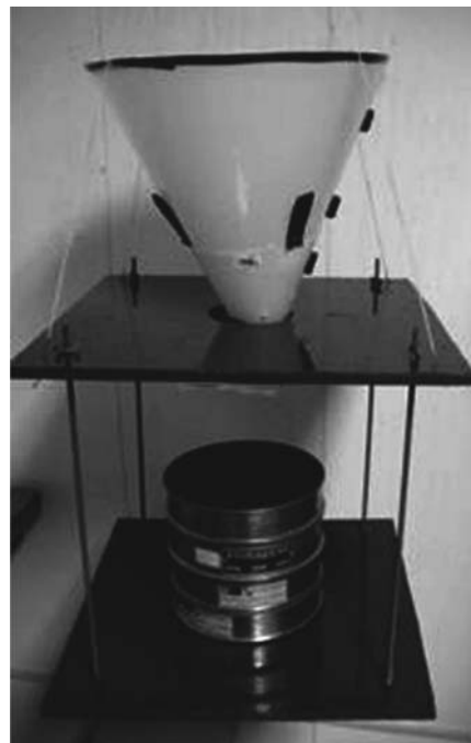
Figure 4 - Pluviation device used for homogenization of the sand before the tests.
