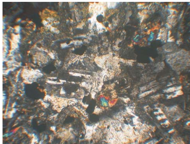
Figure 6 - Photomicrograph showing the intergranular holocrystalline texture of diabase. Labradorite plagioclase crystals occur in laths; pyroxene twinning (taking half of the field) occurs in a few granules among the plagioclase. The polarized light (PL) field width is 1.5 mm.
