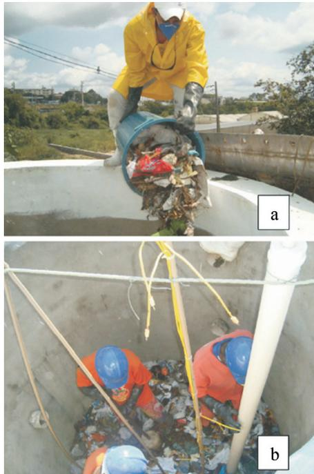
**Figure 3** - a- waste disposal into the lysimeter and d -Waste mass compaction.
