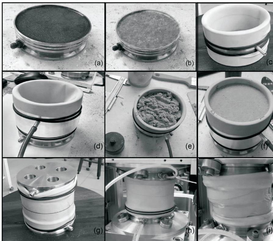
**Figure 5** - Specimen preparation and test procedure: (a) insertion of saturated porous stone on top and bottom cap; (b) placing of saturated filter paper; (c) preparation of latex membrane inside split mold; (d) vacuum application; (e) compaction of soil specimen; (f) finalization of specimen preparation and cleaning of the membrane surface; (g) insertion of the top cap; (h) insertion of specimen on the simple shear apparatus; (i) specimen after shearing.
