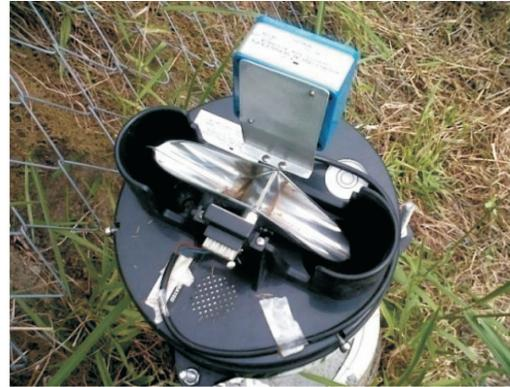
**Figure 7** - Instrumentation: rain gauge installed.
