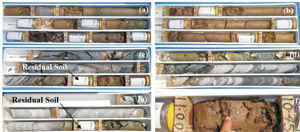
Figure 10 - Drill core samples (a-e), in sequence, from SM-19 (rotary drilling) in Block 4 dam foundation axis. In detail (f) transitional material (soil/rock), depth 10.45 to 11.0 m.
