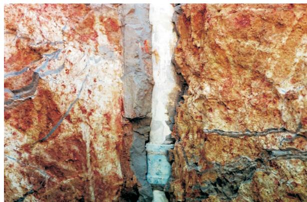
Figure 11 - Inspection trench - Tube a manchette in grouted borehole, with grout planes generated by hydraulic fracturing.
