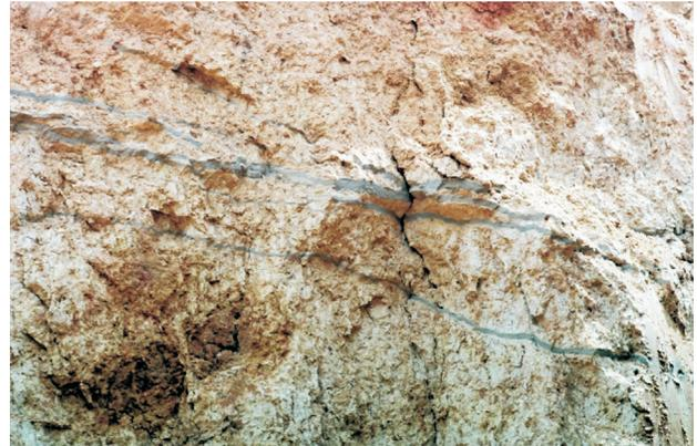
Figure 17 - Inspection trench – clacage planes intersecting and treating canaliculi.
