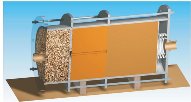
**Figure 13** - Longitudinal section of specimen in a typical CFET (Santos, 2014).
