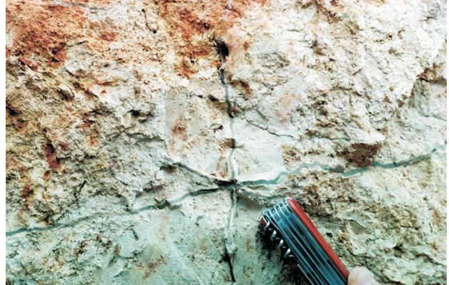
Figure 19 - Inspection trench – treated canaliculi.
