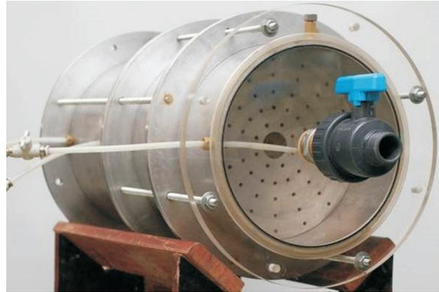
**Figure 9** - LNEC test cell used in the flow limiting erosion test (Santos *et al.*, 2014).
