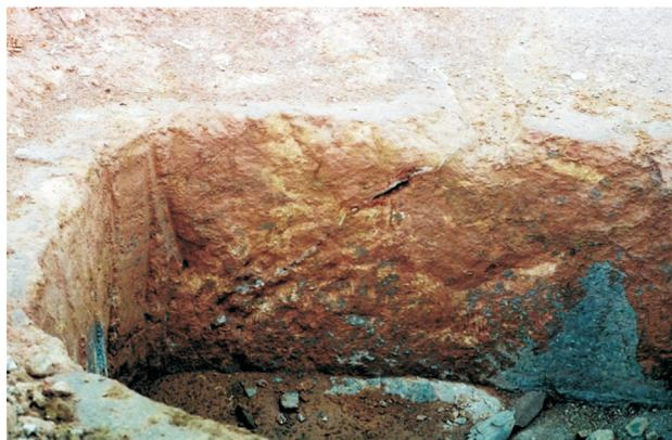
Figure 18 - Inspection trench – clacage planes intersecting and treating canaliculi.
