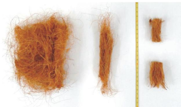
Figure 1 - Coconut fibers 50 mm in length.
