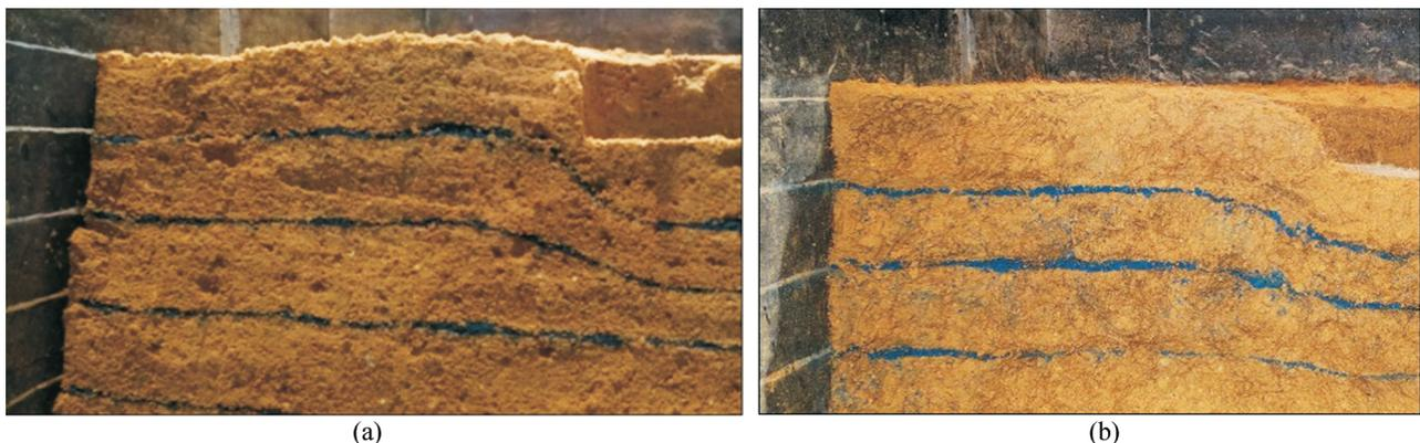
**Figure 8** - Shear mechanism: (a) local shear (non-reinforced sand), (b) punching shear (randomly and layered reinforced sand).
